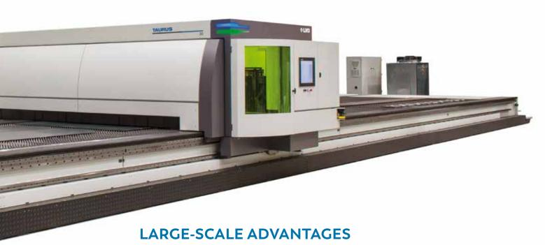
Taurus is a modular system that can be configured to meet your needs. The machine bed length begins at 45 feet (14 m) and can be expanded in increments of 13 feet (4m) to a maximum of 137 feet (42 m). The machine accommodates extra-large or multiple sheets. It improves sheet utilization and nesting efficiency and enables the user to cut parts on one section of table, while loading/unloading on another, keeping downtime to an absolute minimum.
