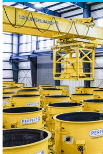
The Magic machine is used worldwide to manufacture both rectangular and circular shaft components in various heights
