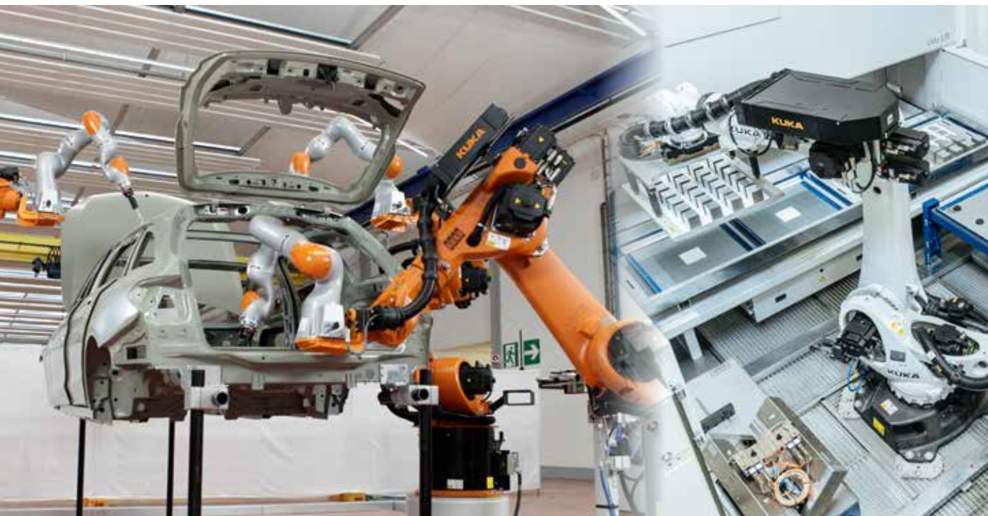
Applying adhesive and sealants to vehicle body
