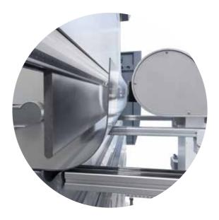
Synchro-Form is a revolutionary new approach to bending XXL profiles, developed by LVD, an industry leader and innovator. The Synchro-Form system evolves LVD's renowned adaptive bending technology to automatically maintain angular consistency and the required geometric profile when bending large parts. Synchro-Form eliminates manual operations, reduces setup and handling, and ensures consistent bending results – delivering high throughput for XXL bending.
