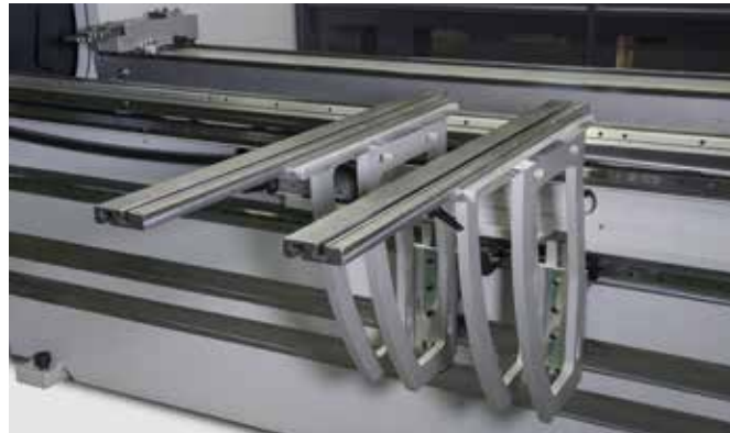
Front supports on guide rails allow quick positioning along the entire length
