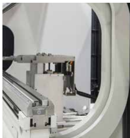
Increase the table-ram/stroke/gap distance in 3.93" (100 mm) steps
