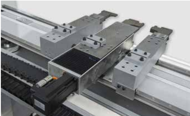
Additional backgauge finger for gauging long parts
