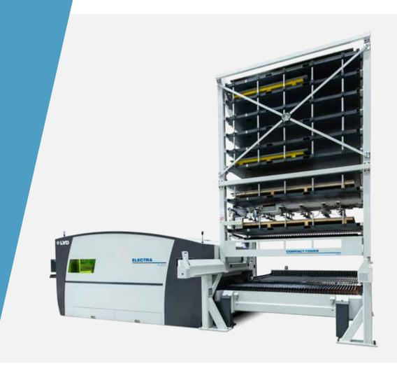
The Compact Tower for Lasers (CT-L) 3015 is a cost-effective tower for loading, unloading and storage of raw materials and finished parts. It is offered in four configurations: 4, 6, 8 or 10 pallets. The system handles  $120^{\circ}$  x  $60^{\circ}$  (3050 x 1525 mm) sheets and material thicknesses up to  $1^{\circ}$  (25 mm) with a pallet storage capacity of 6,600 lbs. (3000 kg). The CT-L unit facilitates unmanned production in a compact footprint.
