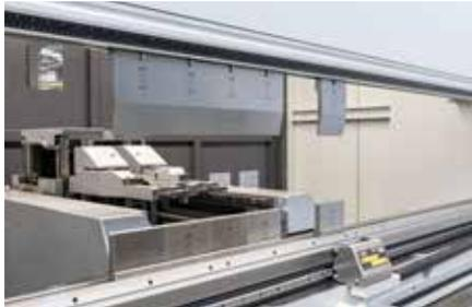
Quick-acting hydraulic clamping installed on the ram.
