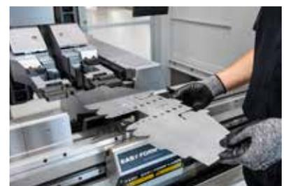
A 6-axis backgauge is automatically positioned for optimum bending results.
