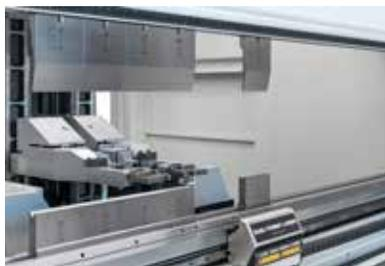
Quick-acting hydraulic clamping is installed on ram and table.
