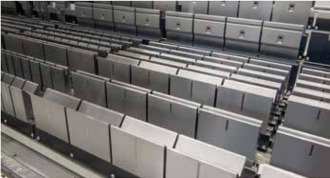
The tooling stadium can be equipped with a flexible tooling configuration to suit specific application requirements: standard punches with a range of radii, as well as V-dies with opening widths from 0.23" (6 mm) to 1.96" (50 mm).
