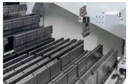
The backgauge with integrated grippers loads and unloads tools for fast changeover and high productivity.
