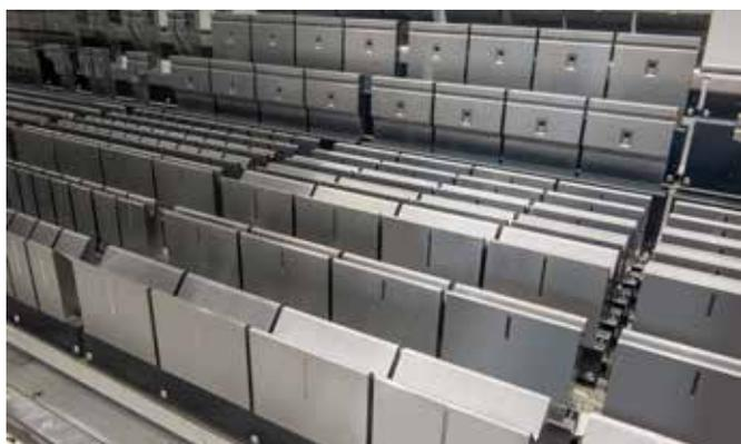
The tooling stadium can be equipped with a flexible tooling configuration to suit specific application requirements: standard punches with a range of radii, as well as V-dies with opening widths from 6 to 50 mm.
