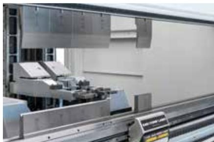
Quick-acting hydraulic clamping installed on the ram.
