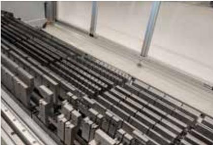
A stadium for two complete lengths of punches and five complete lengths of dies is integrated inside the machine.
