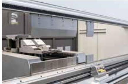
Quick-acting hydraulic clamping installed on the ram.
