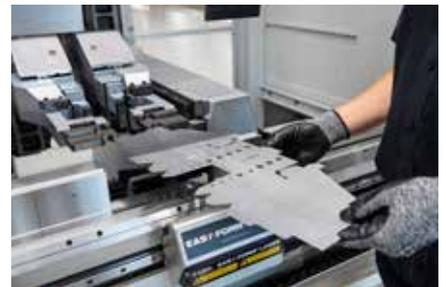
A 6-axis backgauge is automatically positioned for optimum bending results.
