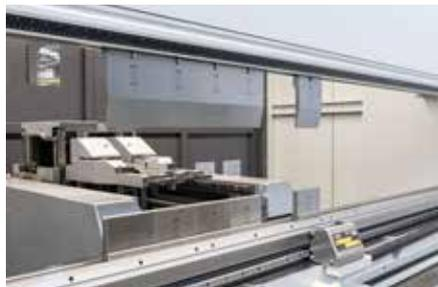
Quick-acting hydraulic clamping installed on the ram.
