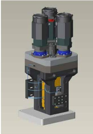
*Elimination of mechanical drive components such as gearboxes makes the electric press easier to maintain.*
