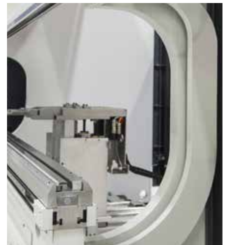
Increased table-ram/stroke/gap distance in 3.93" (100 mm) steps
