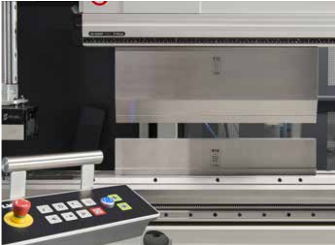
Quick-acting hydraulic clamping on ram and on table
