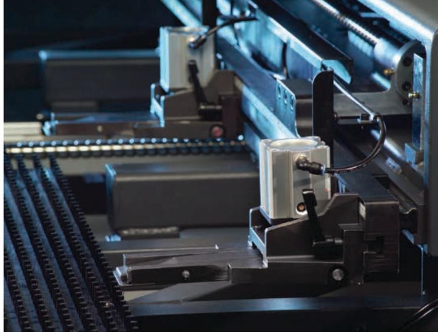
*Smart Clamp minimizes no-punch zones to reduce progressive move requirements and improve material utilization.*
