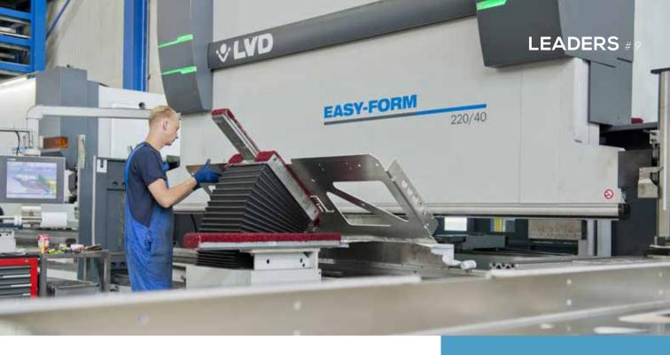
patented Easy-Form® Laser adaptive bending system. Easy-Form performs an in-process measurement which ensures that the desired bend angle is achieved immediately."
