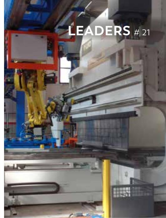
“*Synchro-Form* is a revolutionary adaptive bending system, ideal for making large parts with multiple bends, such as the hexagonal profiles for cranes made by Carpenteria C.S.,” says Andrew Battistini, Sales Director of LVD Italia.
