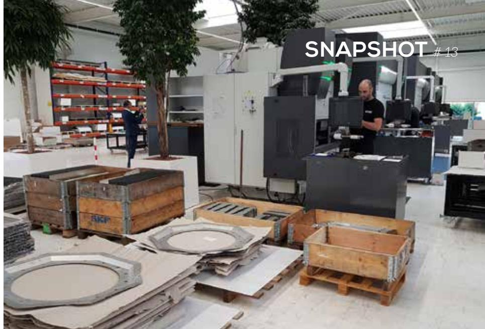
Easy-Form® Laser in-process angle monitoring system ensures the first bend is accurate every time. 24/7TailorSteel also benefits from LVD's CADMAN-B software, which automatically calculates bending solutions and stores them in the CADMAN database to which all LVD press brakes are connected.
