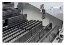
The backgauge with integrated grippers loads and unloads tools for fast changeover and high productivity.
