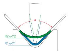
The unique design of the EFL system allows the machine to adapt to material variations such as sheet thickness, strain hardening and grain direction, automatically compensating for any changes.
