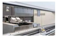
Quick-acting hydraulic clamping installed on the ram.
