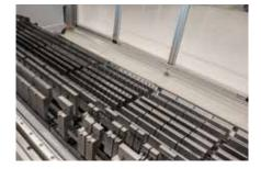
A stadium for two complete lengths of punches and five complete lengths of dies is integrated inside the machine.
