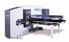
Cost-effective punch press suitable for cellular manufacturing and short production runs
