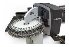
Increased tooling capacity and automatic tool change
