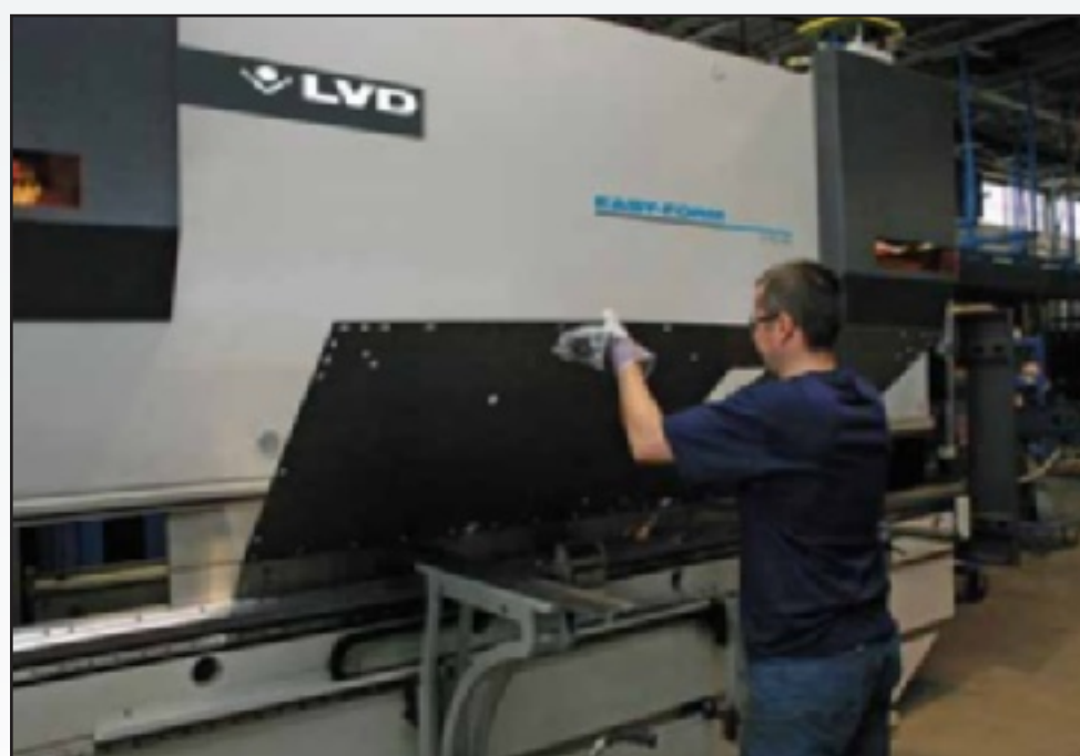
LVD's Easy-Form® press brake advances Delta Elevator's lean manufacturing approach helping to reduce setup times and ensuring accurate bending from the first part.
