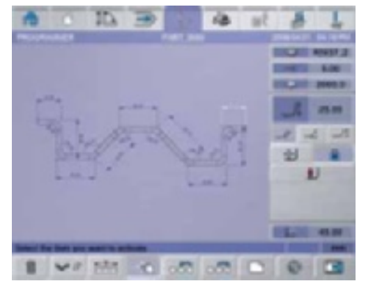
2D and 3D files can be directly imported to the machine control without the need for offline simulation or programming.
